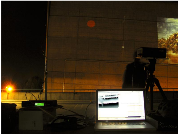
Figure 4. Human Chimes technical layout: Kinect on a telescoping microphone stand, projector, MacBook displaying depth mode screen, and Kyma system.
